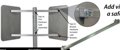
Item # Description Chevron Adjustable Bracket RPBCAB2 Fits 12x18, 18X24 & 24X30 Chevrons Chevron Adjustable Bracket RPBCAB3 Fits 24X30 & 30X36 Chevrons S1824W18(X)A 18" x 24" Chevron Sign S2430W18(X)A 24" x 30" Chevron Sign RPOCG123 12FT • 3LB Galvanized U-Channel Post RHB51625C 5/16" X 2 1/2" Zinc Carriage Bolt RHW516NYLON 5/16" Nylon Washer RHN516VPA 5/16" Breakaway Vandal Proof Nut BA080(X)(XX)0536BMMV 5" x 36" Multi-View Brite-Max Reflector
