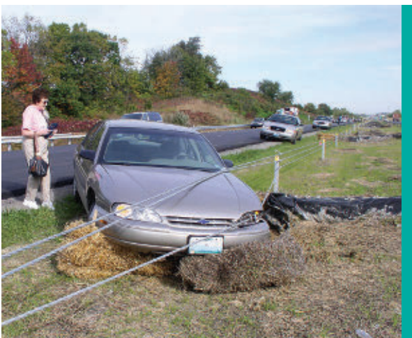
Figure 32. A low-speed crash into a cable barrier system yielded a textbook vehicle capture (Image: Gibraltar)
