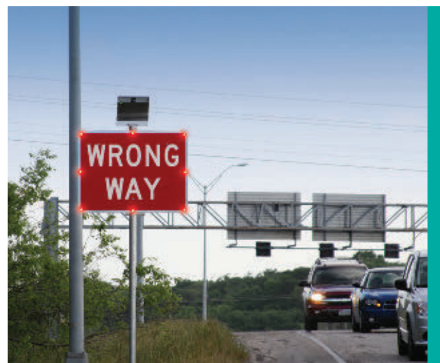
Figure 8. Another use of a Wrong Way sign at the foot of a freeway ramp (Image: TAPCO)
