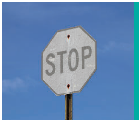
Figure 4. Faded, ineffective signs like this should be replaced to immediately improve roadway safety for motorists (Image: James Scott Baron, ATSSA)
