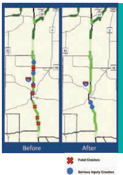
Figure 20. Before-After Crash Reduction on I-35 (Image: MnDOT Office of Traffic, Safety and Technology)
